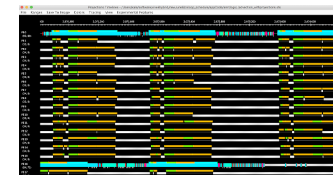
Figure 6: Case Study on AMR: Even though the computational work is well-distributed, the serial portions of the code running on core 0 degrade the performance.
