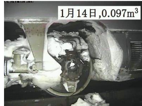
Figure 1: Snow Accretion on Train Bogies [1].
