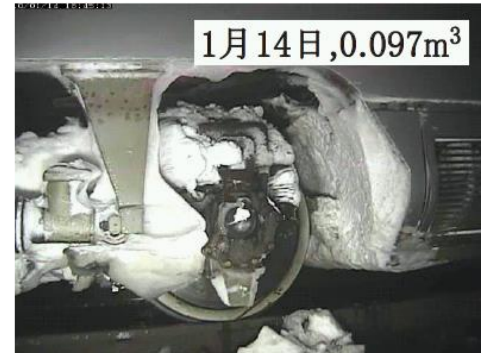
"Snow Accretion on Train Bogies"
