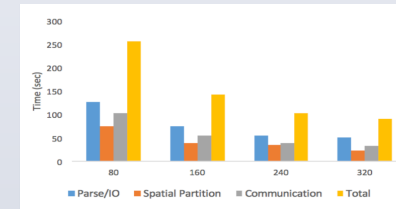
Fig. 8. Execution time breakdown for spatial data partitioning of 137 GB Road network data with 717 million geometries partitioned among 2048 grid cells for different number of MPI processes.
